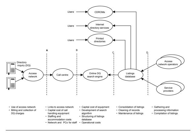
Figure 4.2 The components of a national voice DQ service
